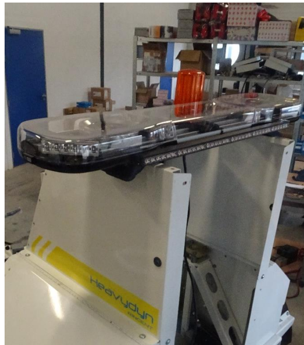
LED ramp with scrolling arrow.
