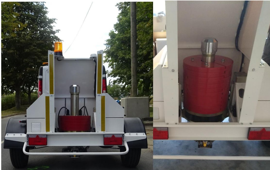
Trailer in FWD configuration (left) and HWD (right)
